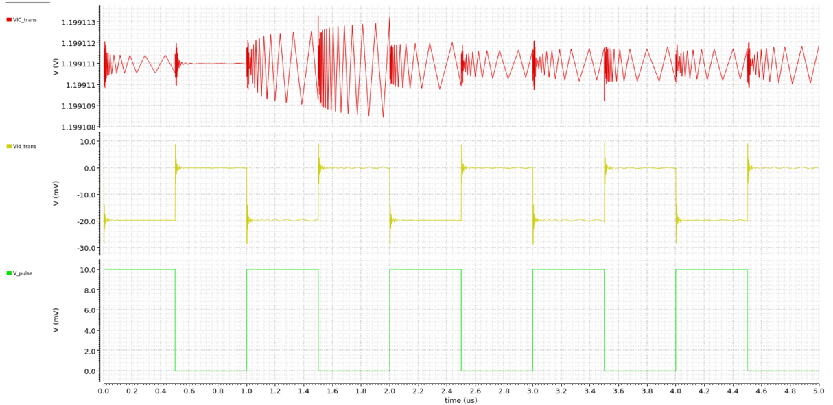
Figure 18: Closed-loop step response of the initial design.
